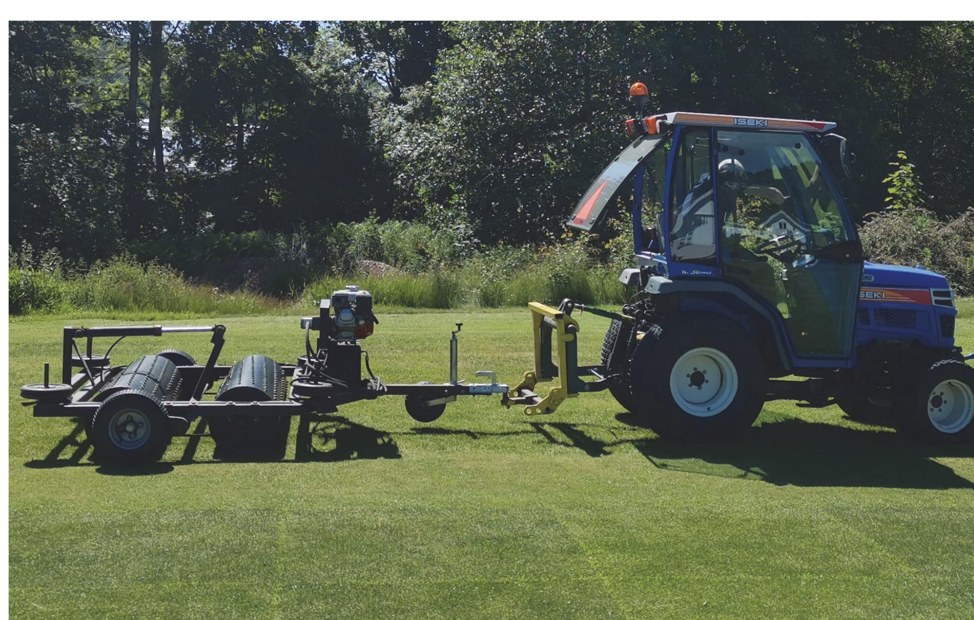
Photo 2. Trailer with two rollers, both with football-shoe studs fixed on the surface, and mounted to a small tractor, used for wear treatments at Landvik. Photo: Lars T. Havstad
